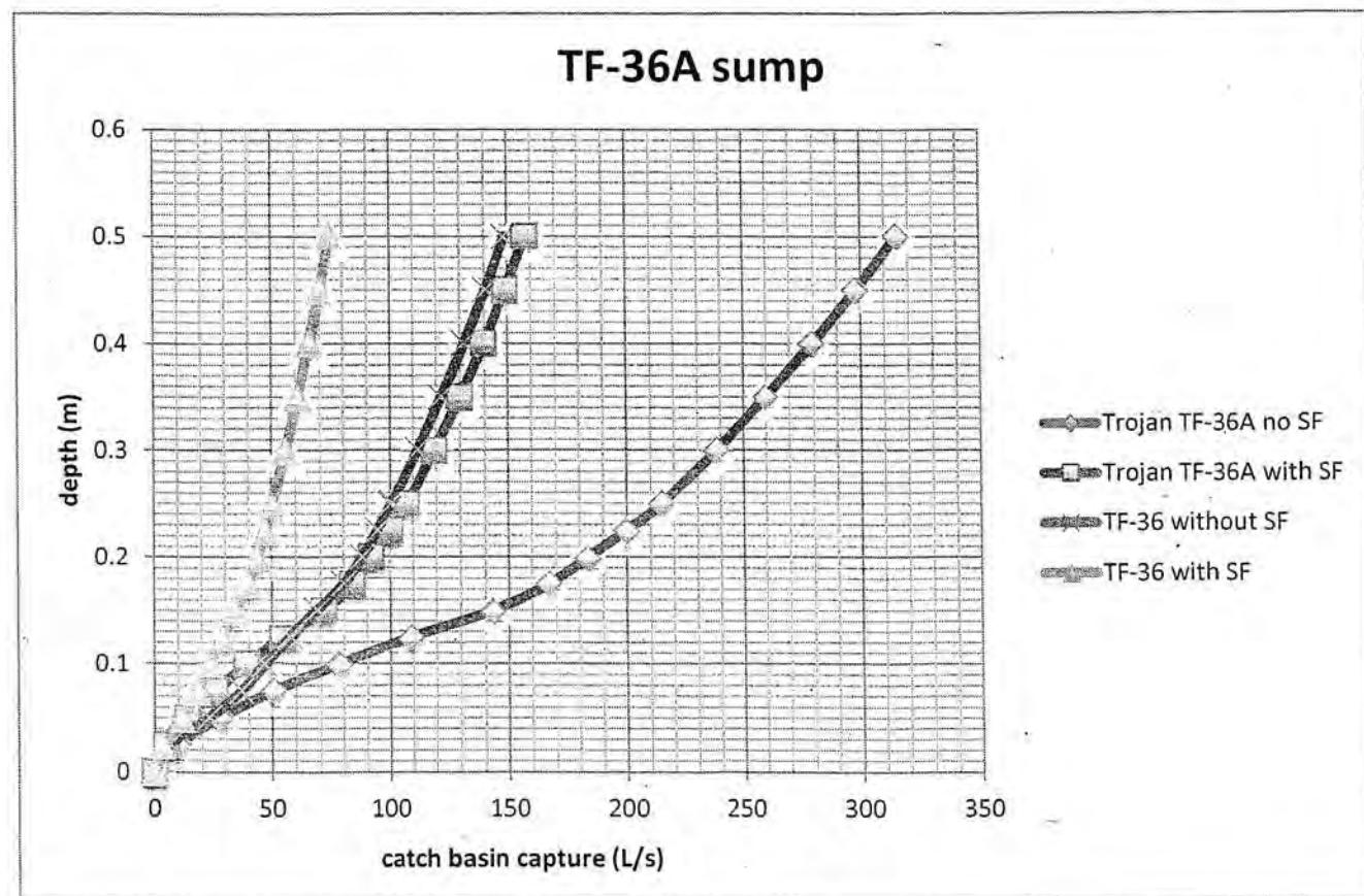
**TROJAN TF-36A Intercepted Flow Rate for Cross Slope 0.015**
