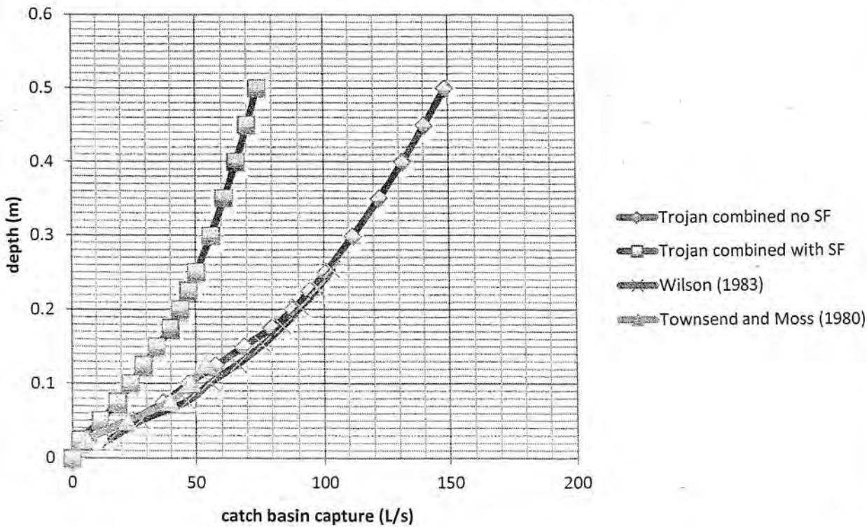
**TROJAN TF-36 Intercepted Flow Rate for Cross Slope 0.015**
